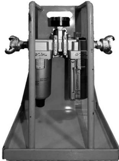
**Fig. 29 Air filter/lubricator unit (air caddy)**
