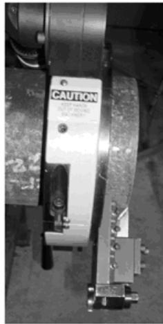
**Fig. 19 Fitting of the beveling tool**
