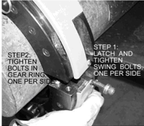
**Fig. 8 Attaching the bottom half of the split frame**
