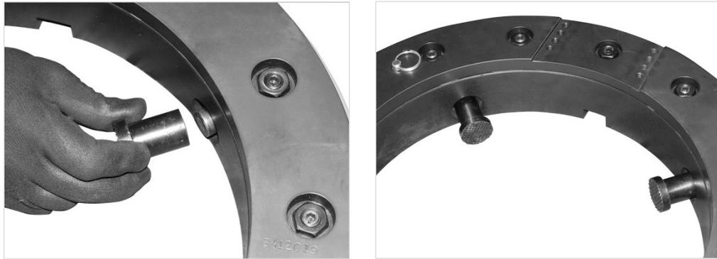
**Fig. 6 Fitting of the locating pads**
