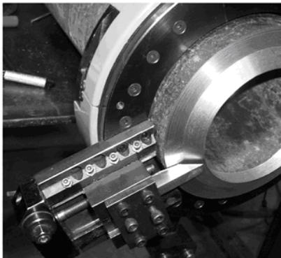
**Fig. 20 Pipe beveling completed**
