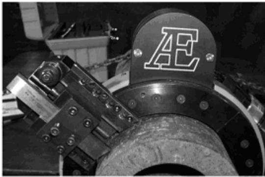
**Fig. 11 Attaching the tool slide**
